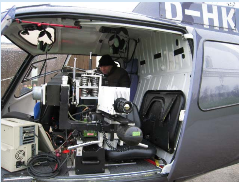
Fig. 8: Measurement technology in the helicopter
