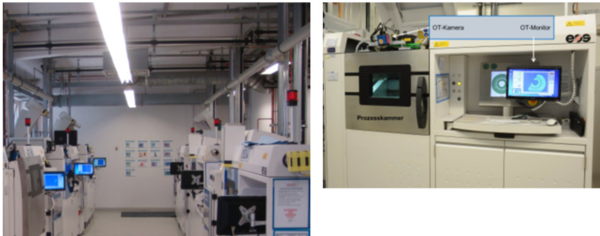
Figure 9: Each AM machine at the MTU Aero Engines machine shop is equipped with a monitoring system
